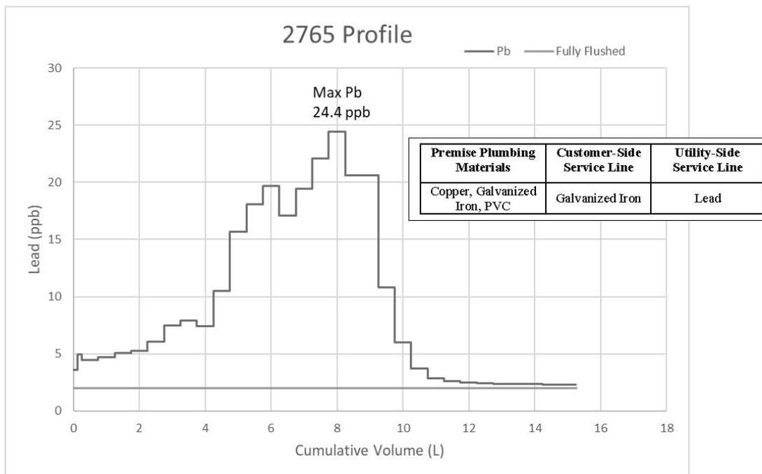
128. This specific plumbing profile consists of copper, galvanized iron, and PVC household plumbing; galvanized iron service on the household side; and lead service line on the water main side. Lead levels increase in the 4<sup>th</sup> liter, where, based on my experience, the household side service line typically begins influencing sequential sample results.
